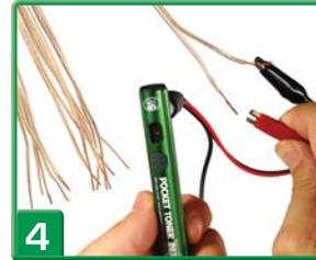
**4** Turn on the NX8 tool and test each of the bare wires at the wire bundle using the alligator clips. Be sure to connect the red clip to the positive wire.
