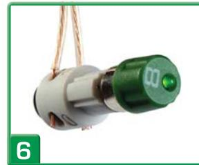
**6** Continuity is also indicated at the ID cap with an LED that lights when it is connected to the NX8.
