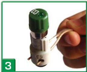
**3** Release the spring-loaded push-button on the 2-wire clip adapter to secures the connection to the wire. This wire is ready to test.
