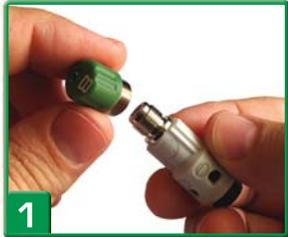
**1** Screw the 8 ID caps onto the appropriate adapters (in this case - the 2-wire clip adapters for testing bare speaker wires).
